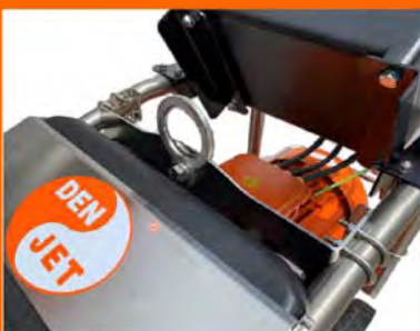
Balanced lifting eye for crane.
