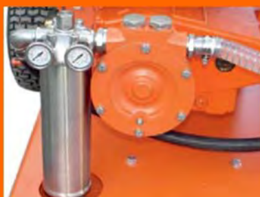
Integrated booster pump & filter systems w. low pressure shut down.
