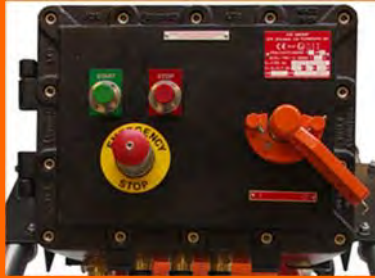
EEx electrical box with main switch, star delta starter & overload relay.
