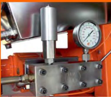
Stainless steel pump-head. Integrated unloader valve.
